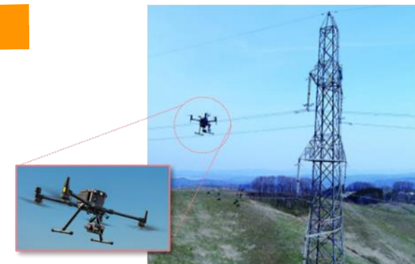
Example of facility inspection utilizing drones (Monitoring of power line deterioration status)
